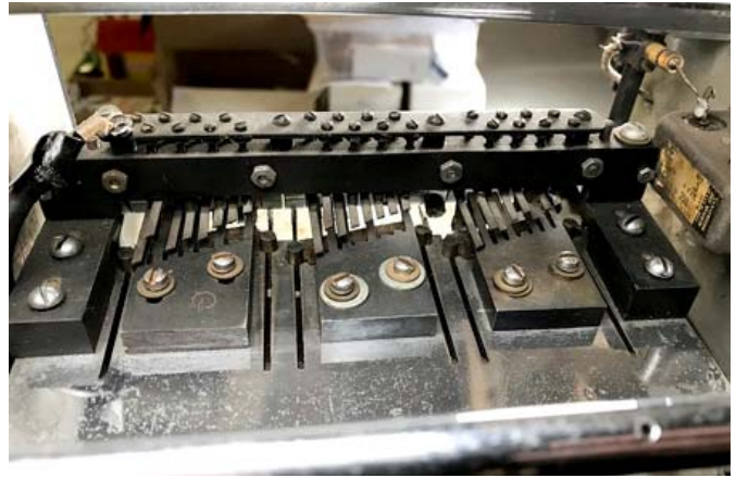
View of the capacitive pickup fingers and three vibrating reed combs. Note several reeds have been broken off.
