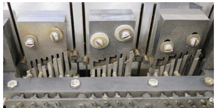
Pick-off reeds shown above the tone reeds.
